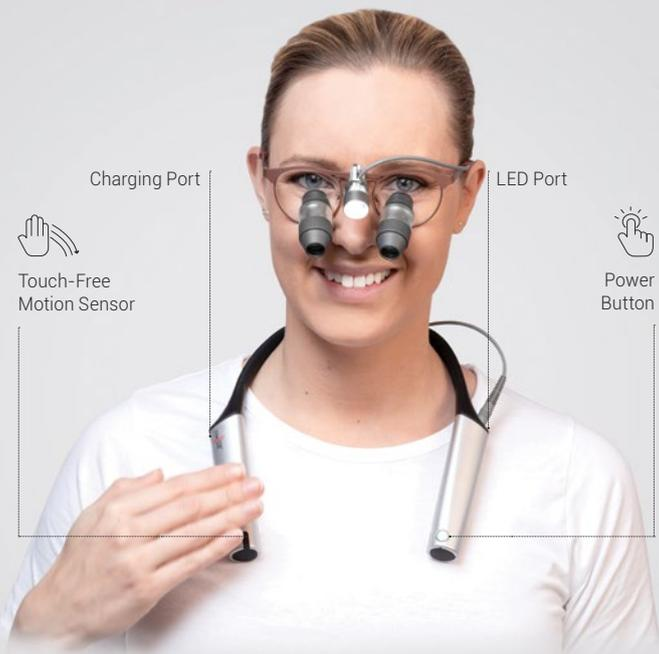
Your PowerBand is a portable control unit equipped with a rechargeable lithium-ion battery.
